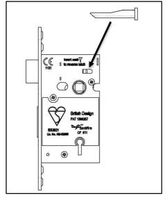
1. Insert 'T' ensuring rounded profile of 'T' matches the profile of hole in the case.
